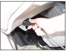
Step 2 Connect the power cable from the AutoLink to the DMI.
