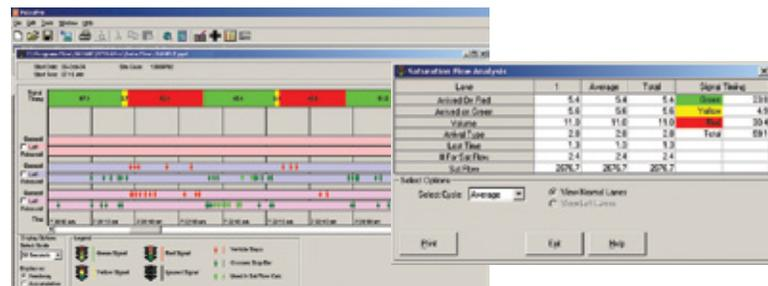
PETRAPro allows you to quickly and easily produce reports for saturation flow rates at intersections. These rates are based on actual real-time data, and not on predefined values that may or may not be accurate. Depending on how the data has been collected in the field, PETRAPro can process and analyze the data for not only Saturation Flow rate, but also vehicle headways, lost times, arrival types, signal timings & approach volumes.
