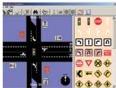
The Intersection Design in PETRA for Windows basically allowed you to configure the lanes of traffic approaching the intersection. With PETRAPro you can enhance this design by placing graphical icons on the intersection. These icons include lane markings, street signs, control devices and data collection locations, as well as the ability to create your own custom icons. You can also add text information to the design.
