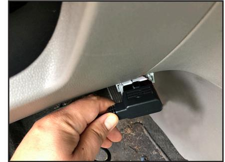
The OBD connector is typically found under your dash near your steering wheel column.
