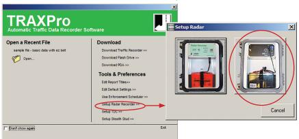
Once the Black Cat Radar Recorder Setup screen appears, you should see a port listed in the COM Port dropdown box at the top as 'Black Cat Traffic Counter'. Click the **Connect** button.
