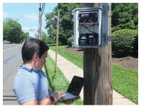
Start the TRAXPro software on your laptop and select **Setup Radar Recorder** from the Tools & Preferences section of the Quick Start screen. You'll then see a screen showing the two models of Radar Recorders. Select the Black Cat Radar Recorder on the right.
