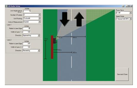
**Unit Height Above Road** – Enter, in inches, how high the Radar is mounted above the road.
