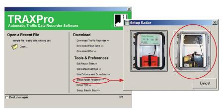
Once the Black Cat Radar Recorder Setup screen appears, you'll see options for COM Port or Remote Site connection. Notice that the Remote Site option is disabled. This is because no sites have yet been created. To connect to a Black Cat remotely, you need to create a Site Listing for the Black Cat in question. To do this, click the *Edit Sites* button and the Site Setup form will appear.
