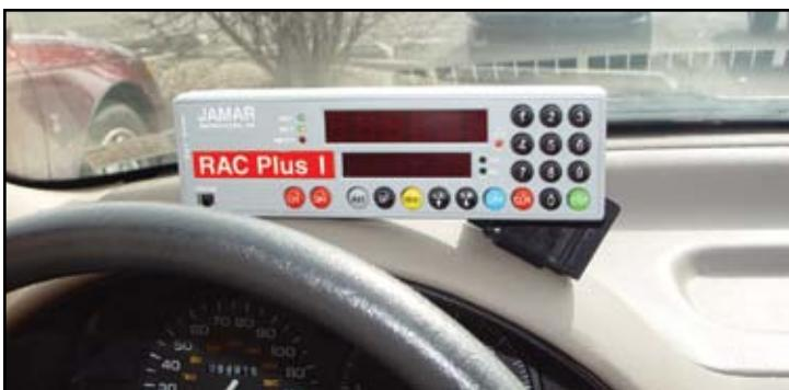
Fig. 2.9 - 'L' Bracket on Curved Dashboard
