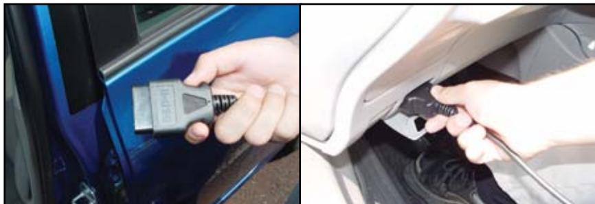
**Fig. 2.1 – Plugging in to the OBD Port**
