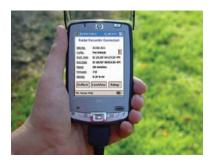
The Radar Recorder Connected screen provides details on the current status of the Radar Recorder. This screen lists the currently entered Site Code, what format of data is being collected (Volume, Binned or Per Vehicle), the start and end date of any data currently in the recorder, the time interval being used to store the data, the current firmware version of the Radar Recorder and the battery voltage level.
