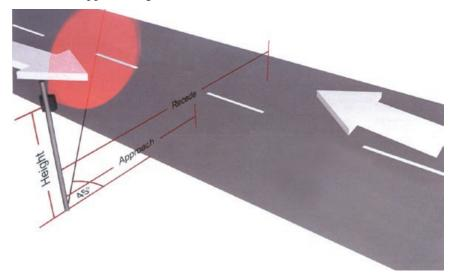
The distance from the Radar Recorder to the middle of the Approach Lane (near side) and the middle of the Recede Lane (far side), should be entered here, as well as the installed height of the Radar Recorder. Note that the lane distances should be measured directly from the pole to the road, as shown above.
