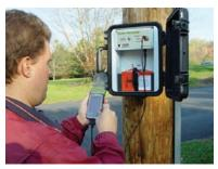
Start the *Pocket Collect* software on your PDA. If the program is able to properly connect to the Radar Recorder, the Radar Recorder Connected Screen will appear.
