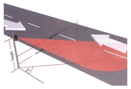
The distance from the Radar Recorder to the middle of the Approach Lane (far side) and the middle of the Recede Lane (near side), should be entered here, as well as the installed height of the Radar Recorder. Note that the lane distances should be measured directly from the pole to the road, as shown above. The distances can be estimates, but should be reasonably accurate to ensure good results.
