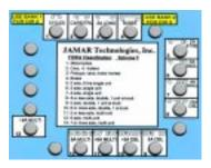
Overlay #1 is used for Classification studies. One side shows the FHWA Scheme F classes, and the other side is designed to allow you to define your own classification scheme. The overlay material allows you to write on it with a pencil or water-based marking pen.
