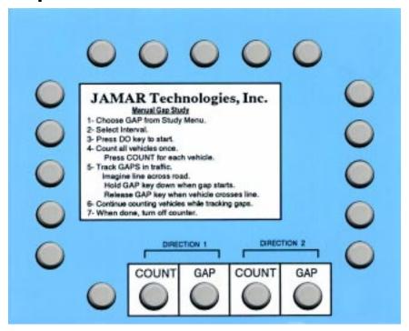
The TDC-8 makes it very simple to do manual gap studies. Most of traffic engineering is involved, one way or another, with managing gaps in traffic. After all, the primary purpose of a signal at an intersection is to artificially create gaps so that traffic can smoothly flow through an intersection. Even though gaps play an essential role in defining traffic patterns, there have been no instruments designed to help manually measure gaps, until the TDC-8.
