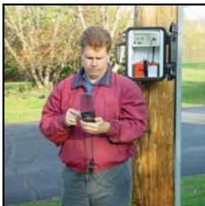
Once the Recorder is setup and recording, the LiveView should be used to check setup accuracy.
