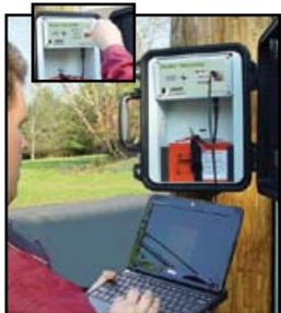
Connect the Interface cable from the computer to the Radar Recorder and start the TRAXPro software.
